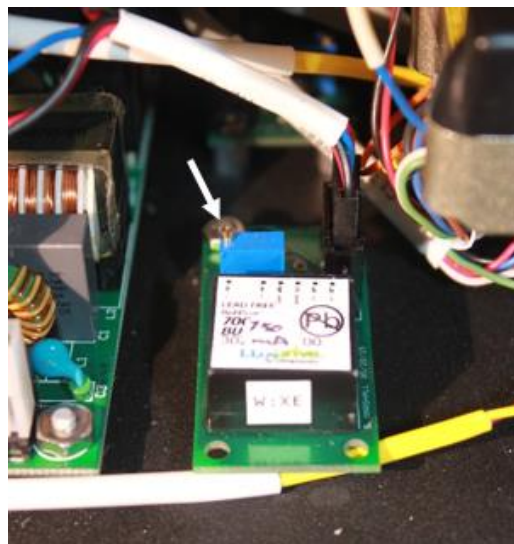
Figure 12: Lamp power supply showing potentiostat
